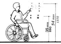
Figure 23b Car Controls Car Control Height
