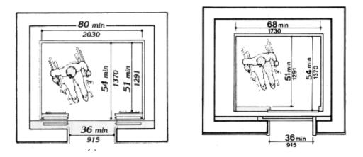
Figure 22 Minimum Dimensions of Elevator Cars
