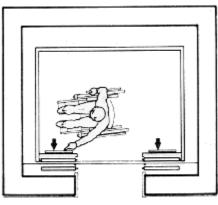
Figure 23c Car Controls Alternate Locations of Panel with Center Opening Door
